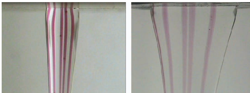
Figure 2 Flow visualization results for colored LDPE layers flowing in the LDPE filament at the die exit under stretching conditions: (a) circular die and (b) slit die. [Color figure can be viewed in the online issue, which is available at wileyonlinelibrary.com .]
